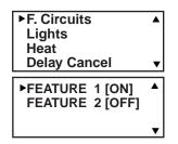
**Right button:** Select the feature circuit to turn ON or OFF. **Up/Down buttons:** Choose assigned feature circuit: FEATURE 1 - 2. **Right button:** Switch the selected feature circuits ON or OFF.
