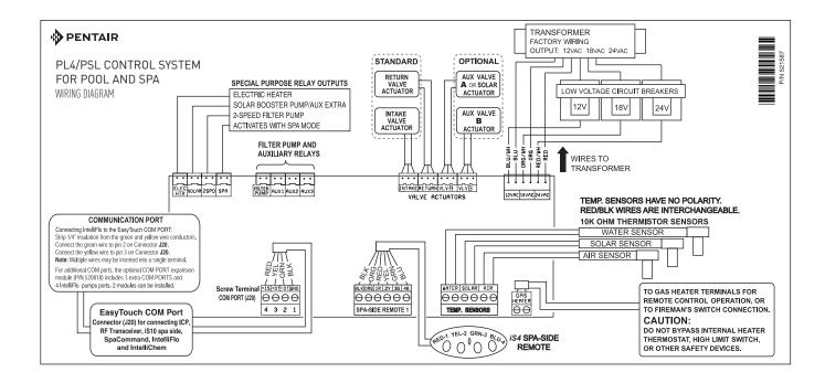
EasyTouch PL4/PSL4 Control System Wiring Diagram (Outdoor Control Panel)
