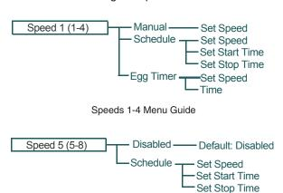
1. Manual: Assigns a speed to one of the four Speed buttons on the control panel. This mode can only be used for speeds 1-4.
