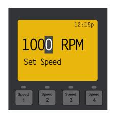
Setting the Anti Freeze Pump Speed
