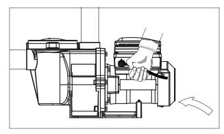
4. Reinstall the RS-485 communication cable.
