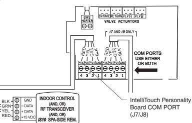
IntelliTouch Control System Circuit Board
